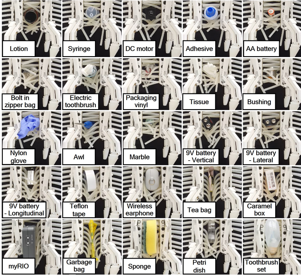
Figure 3.33. Grasping and placing capabilities of the proposed multi-object gripper. Proposed gripper can grasp, store, retrieve and place 23 different objects, including the long cylinders, cubes, cuboids, spherical objects, thin objects, and porous objects.
